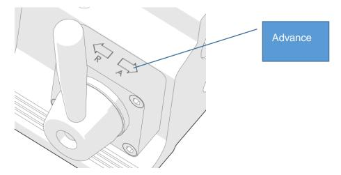
• Pressurise the system by operating the pump handle (2). **Note**: Some pumps emit a high pitched noise during the delivery operation. This is purely the low pressure relief valve venting the unused low pressure oil.
