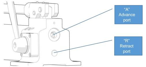
**Note:** Both the advance and return ports on the pump are marked with an "A" and an "R" to identify the ports.
